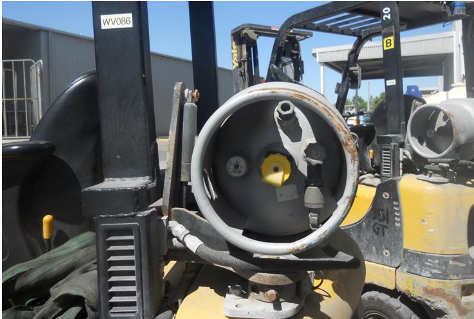
Figure 2 LPG Cylinders Mounted on Two types of Forklifts
