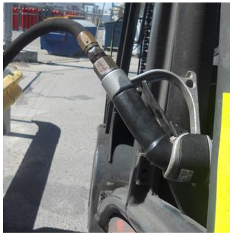
Figure 7 Filler Nozzle Valve Lever Engaged (left) and Disengaged (right)
